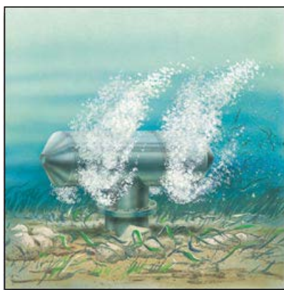
Figure 9-2: Example Wedgewire Screen Installation
